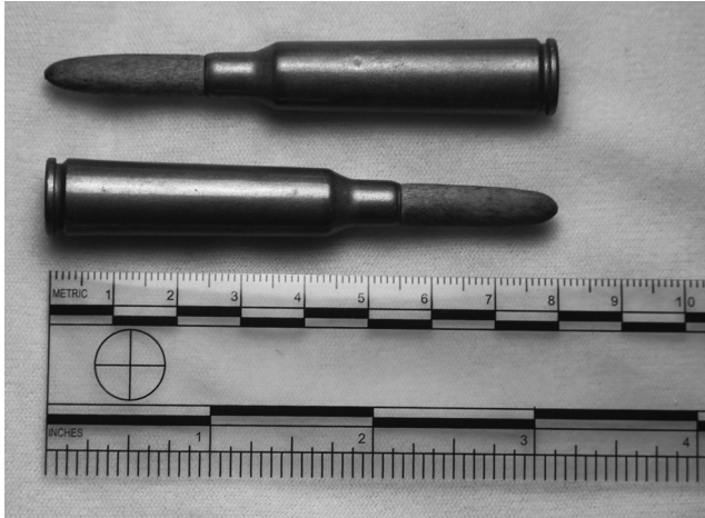
Figure 2.37 (See color insert.) Swedish 6.5mm cartridges loaded with wooden projectiles. (Image from author's collection.)
